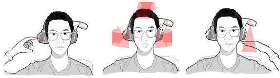
Figure 13: Types of gestures used in this work. Left: touch-based gestures. Middle: user’s head orientation. Right: mid-air gestures.
