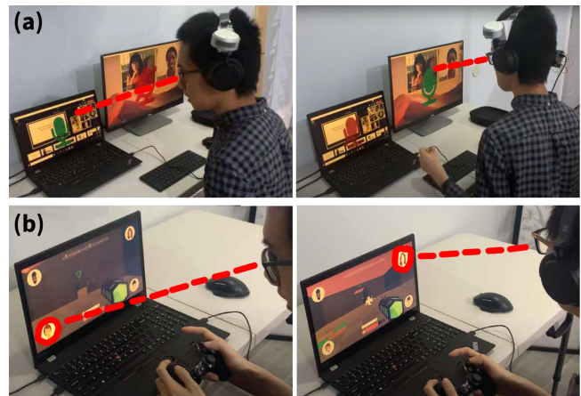
Figure 7: The headphones follow the head-pose of the user, and automatically manage the sharing of video and/or audio between multiple private chats, while communicating availability to other participants in either a) video calling or b) gaming scenarios.
